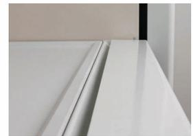
**Flush Sill Airfoil** - Flush with the work surface to provide easy access to the hood interior. Spill trough is designed to provide secondary containment in the event a spill escapes the primary containment worktop. Air foil is hinged for easy cleaning.
