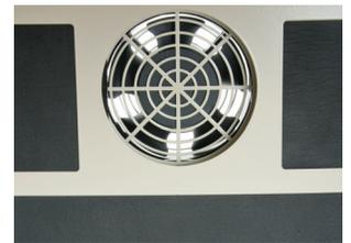
**Cooling Fans** - Optional internal fan to ensure adequate air cooling is provided to the pump. Fans pull fresh air in through the door louvers and blow heated air out behind the cabinet or into building ductwork. Fan plugs into switch controlled outlet.
