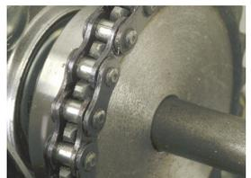
**Chain Drive Sash** - Chain and sprocket mechanism that delivers the easiest and most reliable sash operation available with an exceptionally long life span.
